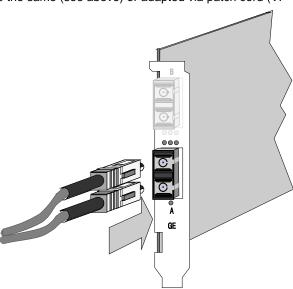
Figure 2. Connecting fiberoptic cables/connectors
